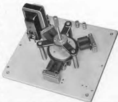
FIGURE 3. The motor assembly which may be employed to drive discs, contactors, and small generators
