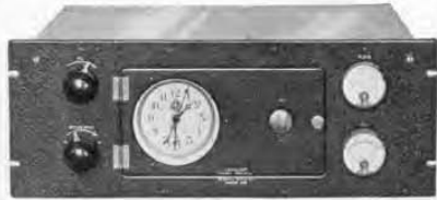
FIGURE 5. The clock and an amplifier may be assembled in one unit and used for relay-rack mounting
