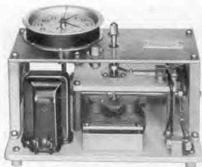
FIGURE 6. This clock designed to run on 60-cycle circuit has both a seconds and 0.1 second contactor
